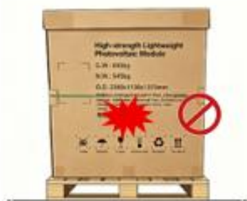
No impact on the container
